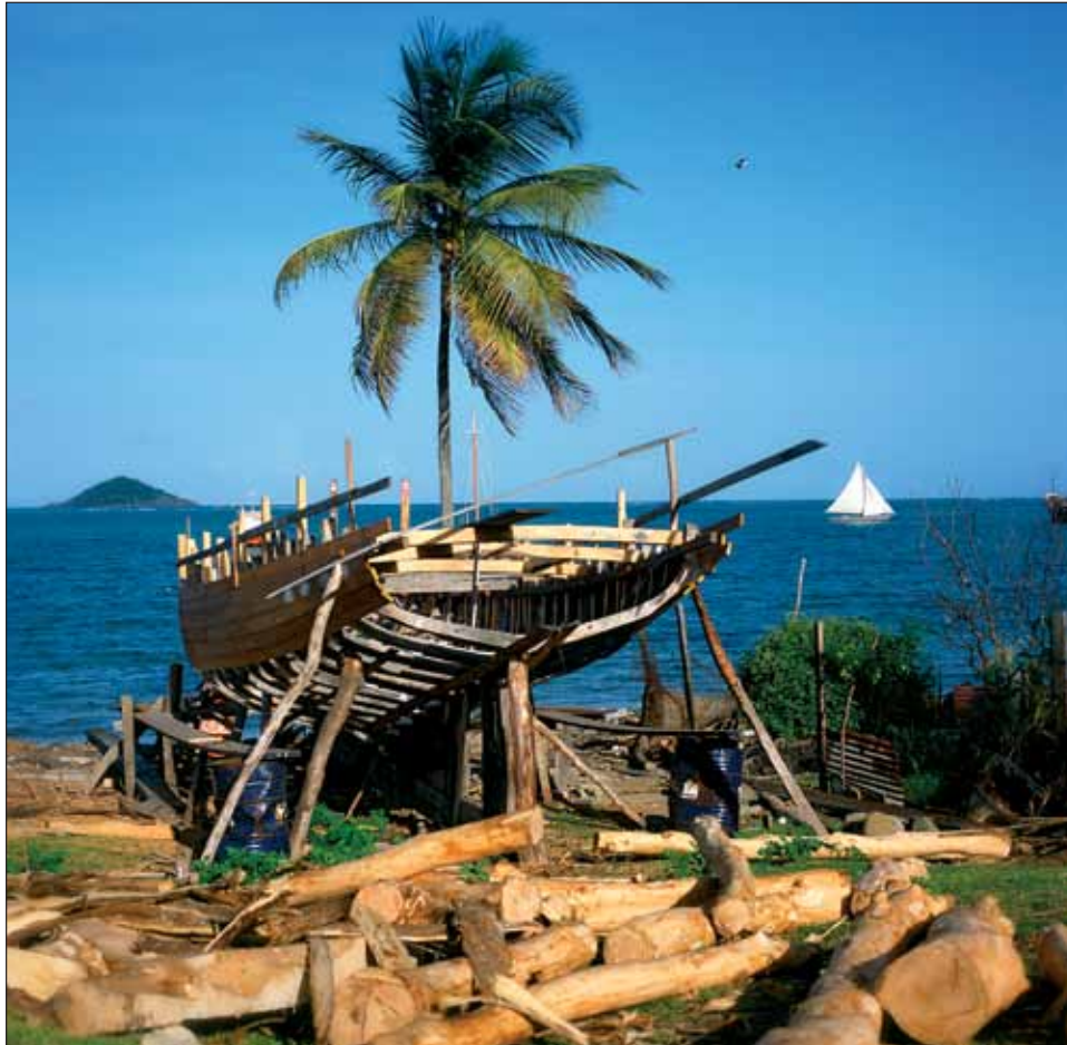
GENESIS in frame, 2003. "During the build," writes Alexis Andrews in the book Genesis , "GENESIS was exposed to the elements. Over a period of 17 months the sun baked her, the rain soaked her, and the wind howled through her ribs."
